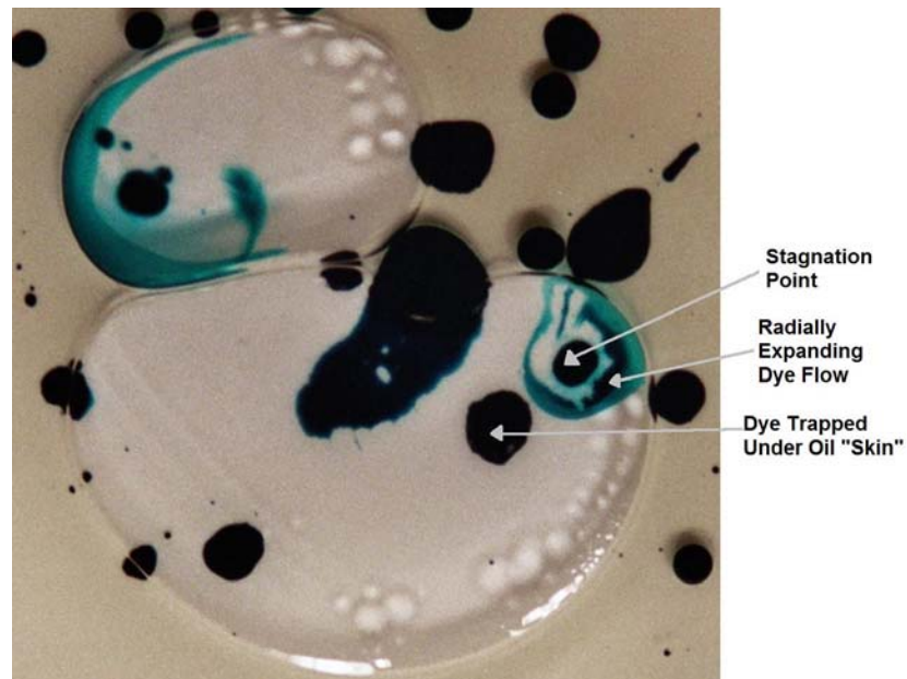
Figure 4: Dye and water interaction showing stagnation point flow and radially expanding jet
