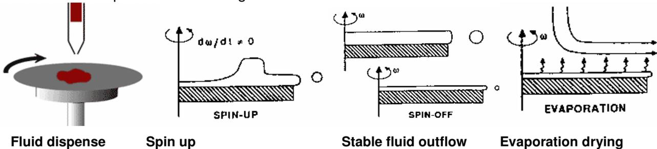
A spin coating model was published by Emslie, Bonner, and Peck [J. Appl. Phys. 29 (1958) 858-862] assuming that a Newtonian non-volatile flow has reached a stable condition where the centrifugal and viscous forces are just in balance (as shown in stage 3). When the centrifugal and viscous forces are in balance, the governing equation and film thickness as a function of material can be shown
