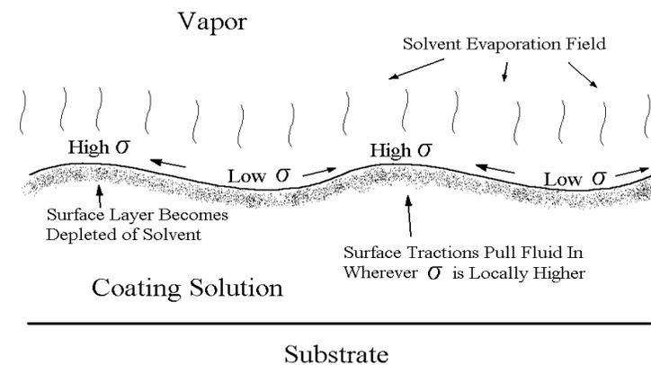
During hot plate baking, the early evaporation of light solvents can cause an enrichment of water and/or other less volatile species in the surface layer. If, the surface tension of this layer is larger than the starting solution (and what still exists at deeper levels), then instability exists where the higher surface tension actually draws material in at regular intervals and the spaces in-between are more able to evaporate, and surface relief develops.
