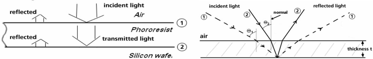
**Figure 2** Light incident to transparent thin film and the path difference of light.
