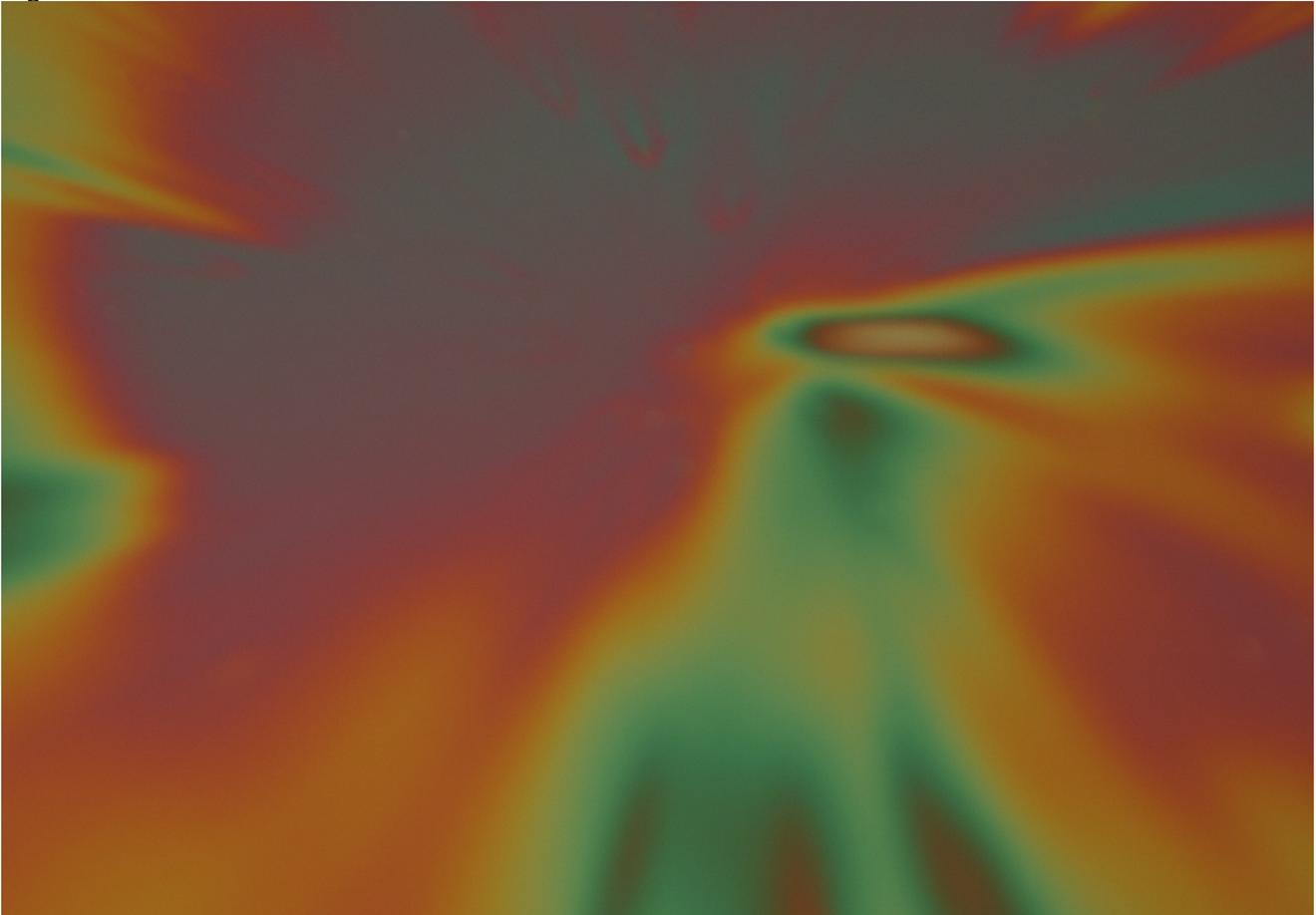
**Figure 1 A non-uniform coating on silicon wafer shows iridescent colors.**
