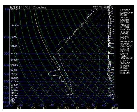
When looking at the 6pm Skew-T plot we can see that the neighbor line is nearly matching the parcel line from approximately 4000m to 8000m. This means that the clouds could be forming due to the borderline instability, this observation is confirmed by the cape of 24, which has increased from a cape of 19 earlier in the morning. This pattern shows us that as the day progressed clouds should have been forming, and my image captured this formation approximately half way through the formation.
