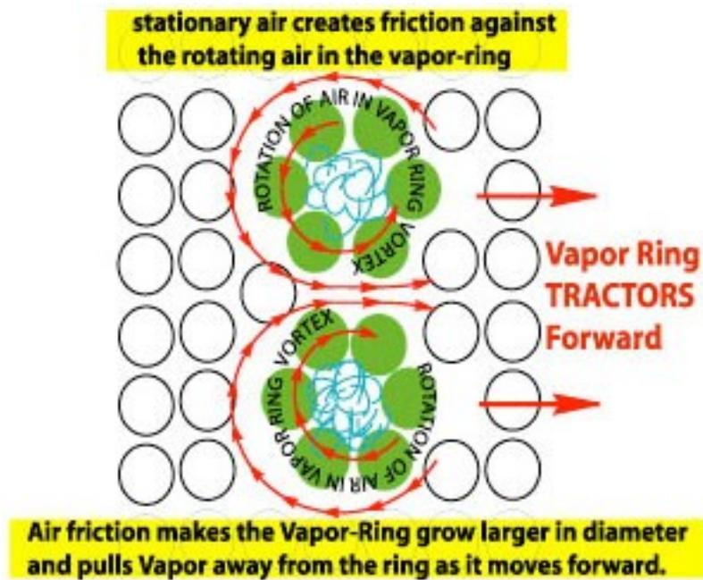
Figure 2: Vortex ring motion explained
