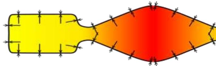
The net thrust of a rocket can be determined by this equation:  $F = \dot{m}V_r + A_r(P_r + P_{atm})$  (Barbarika). This equation is the mass flow of the gas exhaust times by the actual jet velocity of the exit with the flow area of the nozzle times by the different of the thrust pressure and the atmospheric pressure.
