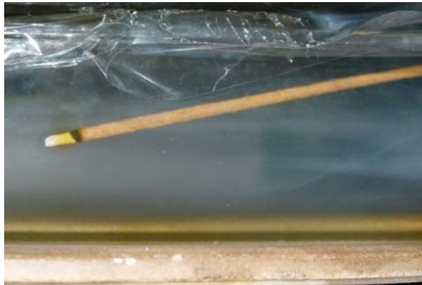
Figure 1. Experiment photo of incense smoke used to visualize convecting air cells between two parallel plates.
