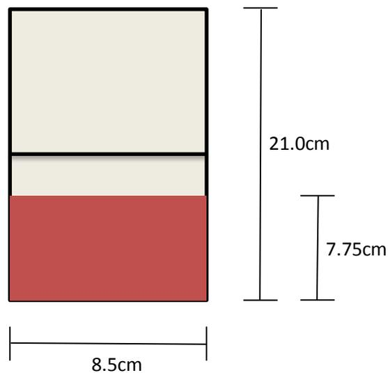
The height of the ooze tube is 21.0cm, the width is 8.04cm, and the height of the fluid settled is 7.95cm. The ooze tube is made of acrylic with approximately .2cm thick walls. The weight of the entire ooze tube is 491.8g. With all these dimensions and assuming the density of acrylic is  $.9\text{g/cm}^3$  we can estimate the density of the fluid inside. First let's calculate the weight of the acrylic used in the ooze tube.
