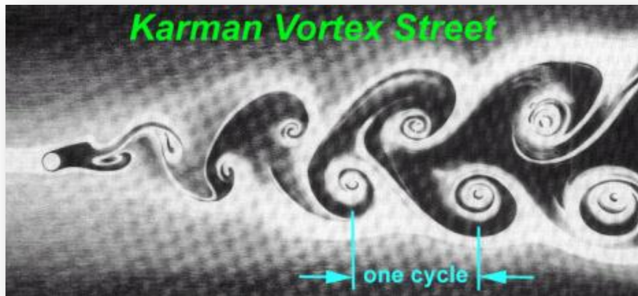
Figure 1 Example of Karman Vortex Shedding 1
