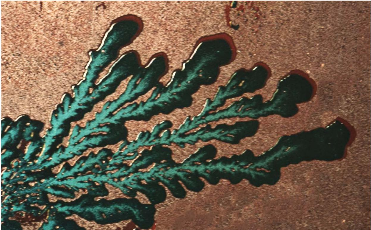
This is the third flow visualization submittal for the MCEN 4151 class. The image was taken individually, however a group was assigned to help with the brainstorming ideas for the photo, the setup, and the lighting of the image. The phenomenon that was intended to be observed was the Hele-Shaw flow fingering between two pieces of glass. Team members that helped to make this photo possible include; Coulter Pohlman, Hans Loewenheath, James Shefchik, and Spencer Aguilar.
