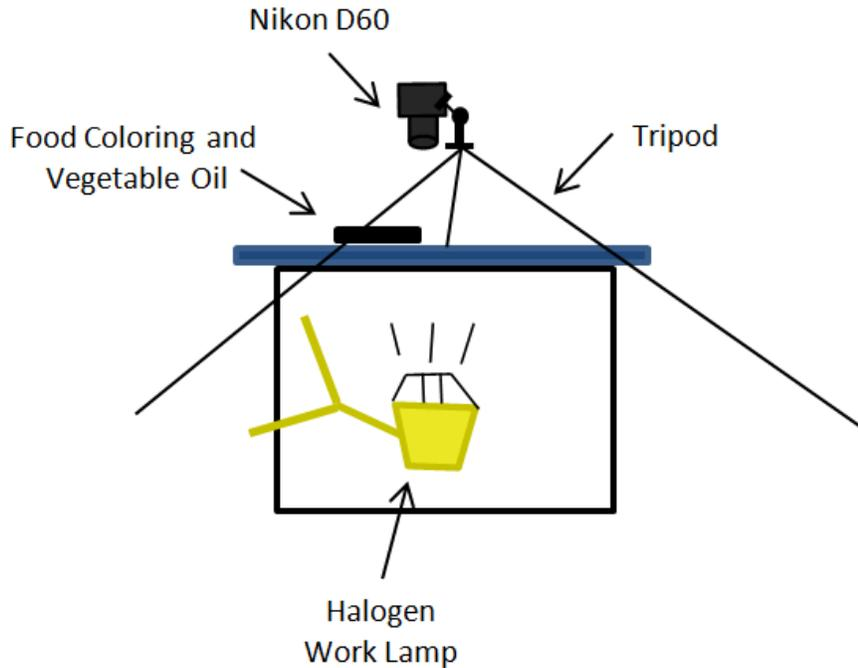
**Figure 1. Photo Apparatus**
