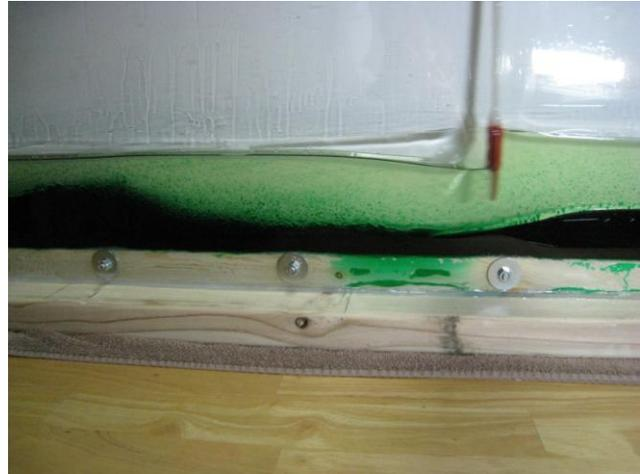
**Figure 3: Spatula disturbing the upper layer of fluid**
