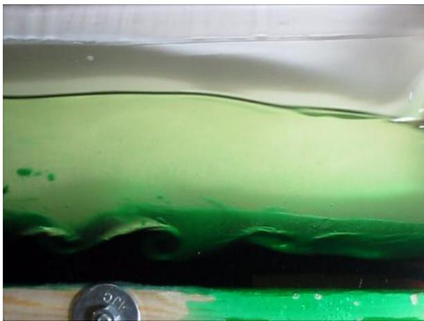
**Figure 4: Kelvin-Helmholtz instability in the channel**
