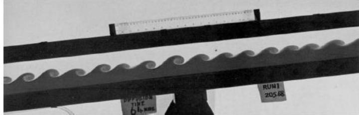
**Figure 1: Kelvin-Helmholtz instability experiment<sup>1</sup>**
