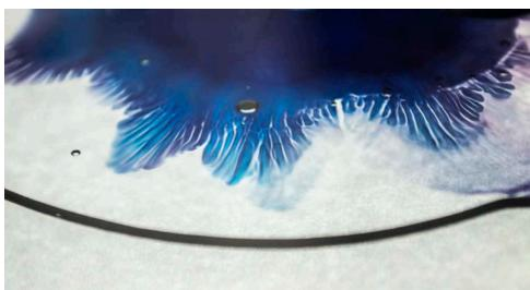
We instead created them from another angle. After injecting a red water sample into the blue, we slowly lifted one plane of the cell. This introduced suction in the cell. Air rushed in from the sides, and the water formed veins where the air didn't go.
