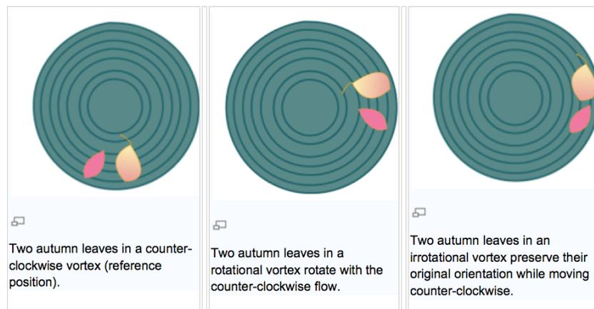
Figure 3: Example of the difference between rotational and irrotational vortices. [Golin]
