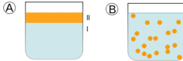
Figure 1: A. Two immiscible liquids. B. An emulsion of Phase II dispersed in Phase I. [Emulsion]
