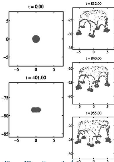
Figure 3 Drop Separation<sup>4</sup>
