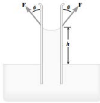
Figure 3: Adhesive forces causing capillarity 3
