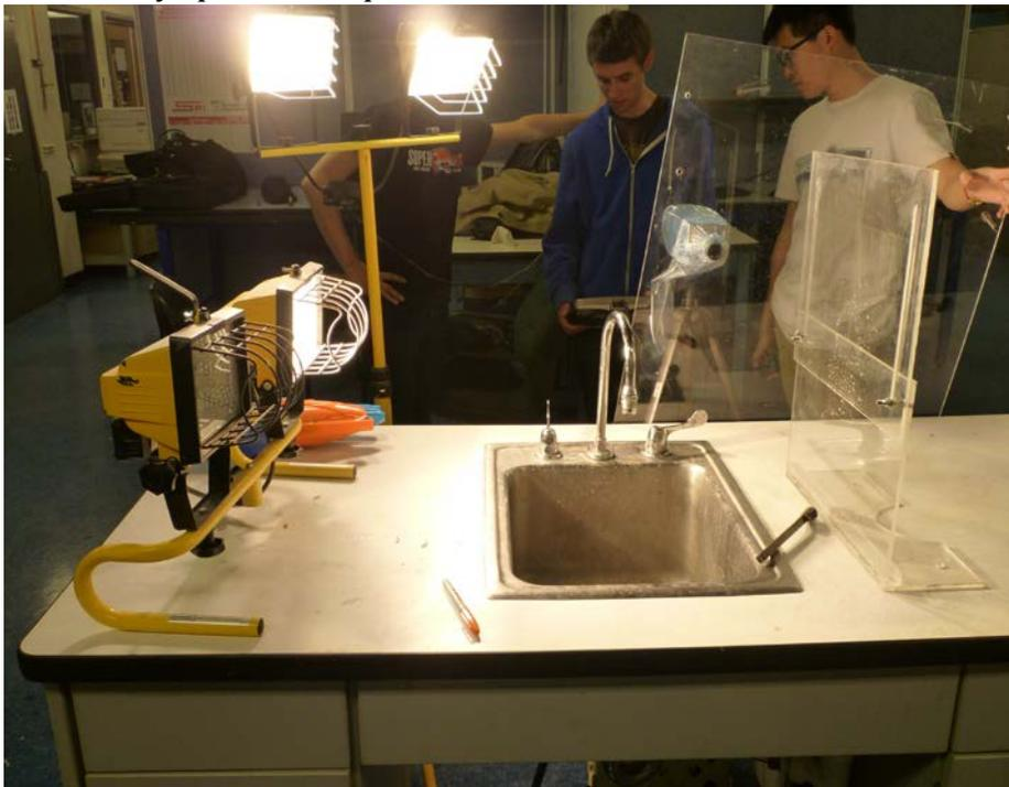
sheet to provide a barrier between the camera and the pool of water. These two pieces ensured that the camera would remain safe even with the large splashes of water observed with the one-inch bolt. The bolt was dropped from approximately 12 inches above the pool of water. The head was held downward in order to ensure the impact was with the head of the bolt as seen in the video.
