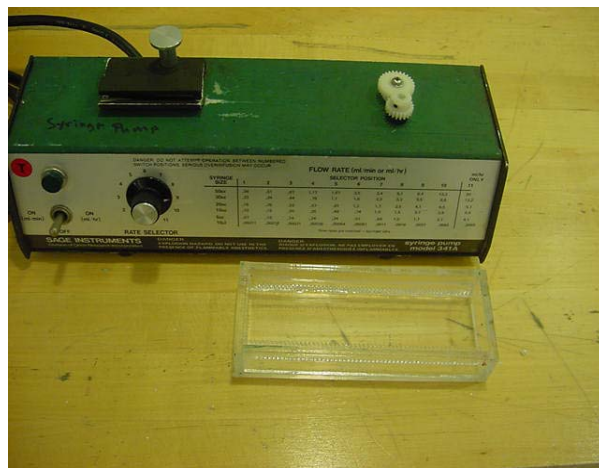
Figure 6-a: syringe pump – gears (top) with gear racked box
