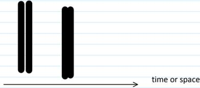
Resolution = minimum distance between two objects for them to be recognized as separate.
