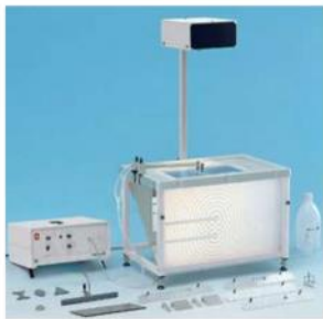
8) Surface gravity waves with a shallow water ripple shadowgraph imagery. Can visualize wave: interference reflection refraction dispersion
