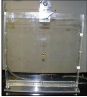
7) Capillary waves - visualization using a view graph projector.
