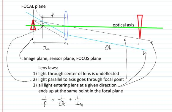
As object moves closer, lens must move away from sensor plane to maintain focus. Mechanical limit defines near focus distance. For a given object distance, as the lens becomes shorter, the image distance (flange standoff?) also gets smaller: hence smaller cameras do well for macros
