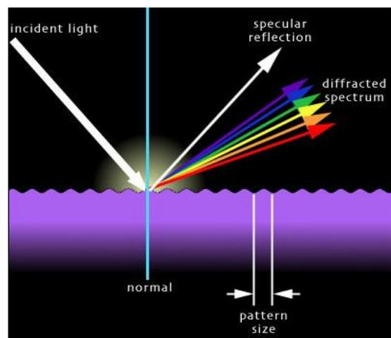
Figure 3: Surface Roughness Causes Diffraction, courtesy of <http://emerald.tufts.edu/>
