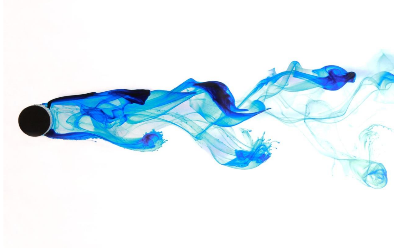
Figure 6: Karman vortex street behind a cylinder in water
