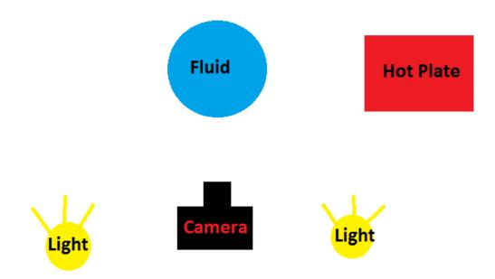
The visualization techniques used are very straight forward. A clear beaker hold water and a camera is able to see into the water and capture it's flow patterns. Two fluorescent lights overhead were used to illuminate the water, giving good contrast when looking at the ripples.
