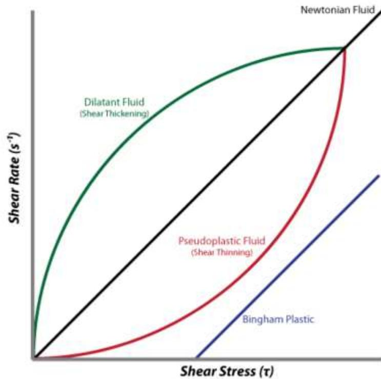
Figure 1: Shear Rate vs. Shear Stress Plot
