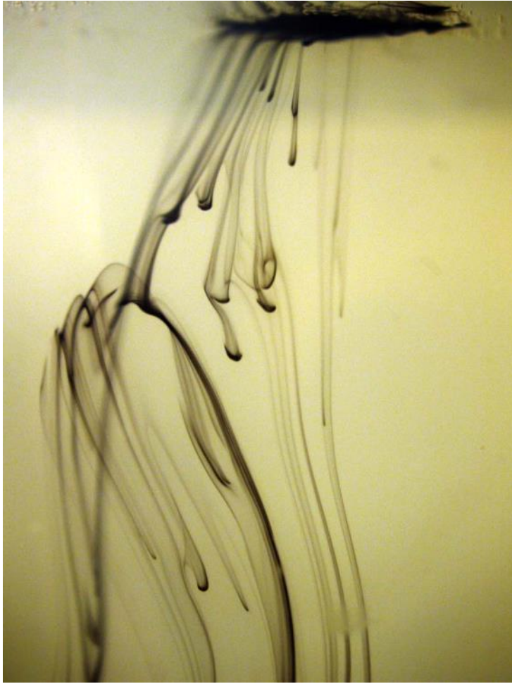
India ink falling through water shows the Rayleigh-Taylor instability. Gordon Browning. Get Wet Fall 07.
