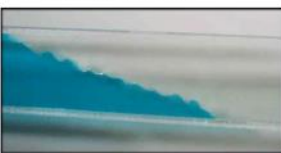
Example of a gravity current with two layer tank. Kelvin-Helmholz instability in a 6' clear acrylic tank –two or three layer - dye visualization
