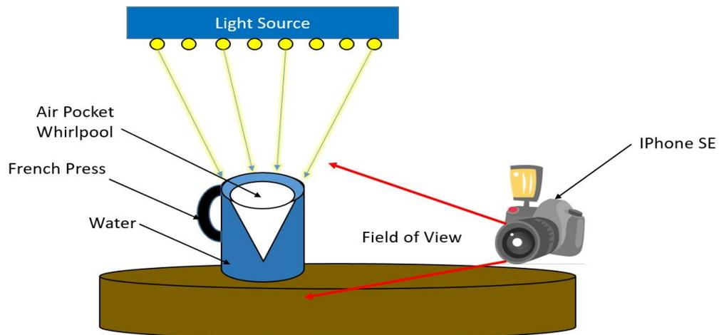
**Fig 1.** The apparatus set up after the spoon is removed from the french press
