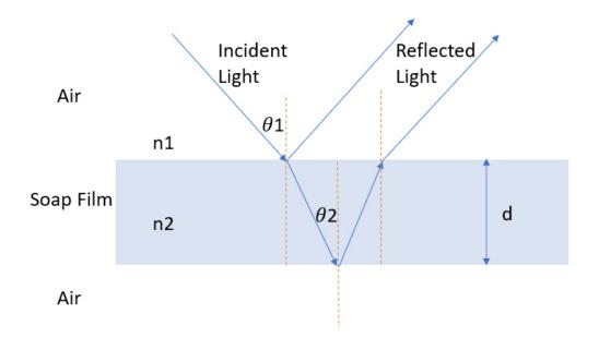
Figure 1: Effect of Index of Refraction
