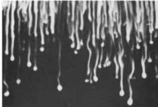
Salinity and temperature diffusion rate differences result in vertical mixing within a statically stable fluid.
