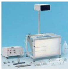
7) Surface gravity waves with a shallow water ripple shadowgraph imagery. Can visualize wave: interference reflection refraction dispersion group and phase velocity plane and circular waves Doppler effect 8) Thermal convection - aluminum flake visualization of convection over a heating pad in a 6" layer of silicone oil
