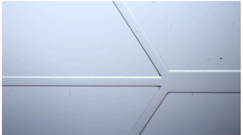
The microfluidic device sits atop the stage of the fluorescence microscope, with an optical path as shown in **Figure 3**. Unlike with traditional optical microscopes, light from this microscope's 400 mW LED light source passes *through* the sample ( $D_{LED\ to\ Object} = 600\ mm$ ) to the viewing optics, or in this case, a DSLR camera.
