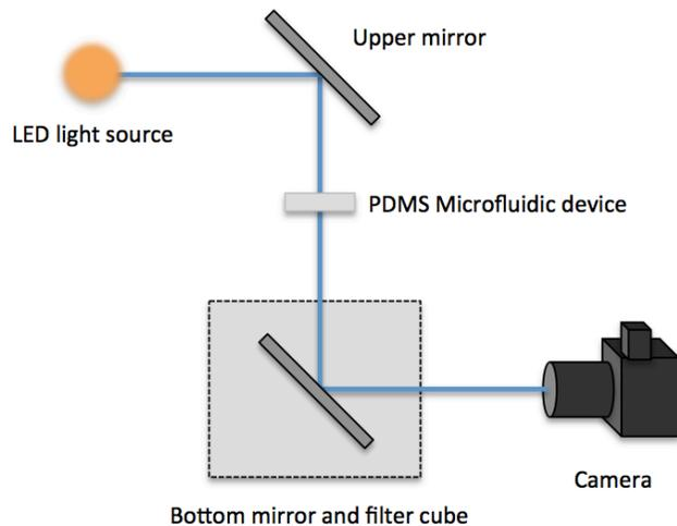
**Figure 3.** Optical path and simplified setup of the fluorescence microscope, showing how light passes through the sample, rather than being reflected off of its surface.
