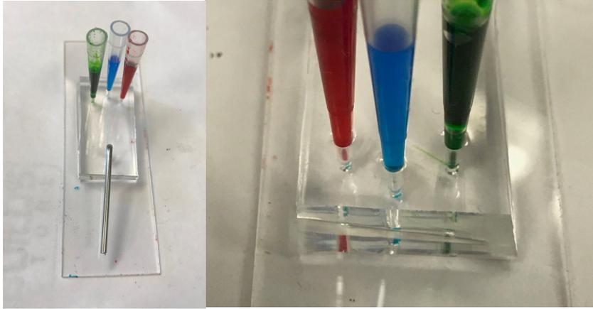
**Figure 1.** The microfluidic device used in this experiment. At left is the entire microfluidic device (PDMS on a glass slide), with three pipette-tip reservoirs filled with the dyes and a bent metal collection tube. At right some of the green dye can be seen running through its channel.
