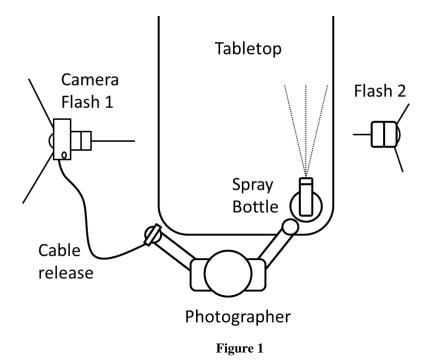
This figure shows the approximate arrangement of the camera, flashes, photographer, and spray bottle used to take the picture.
