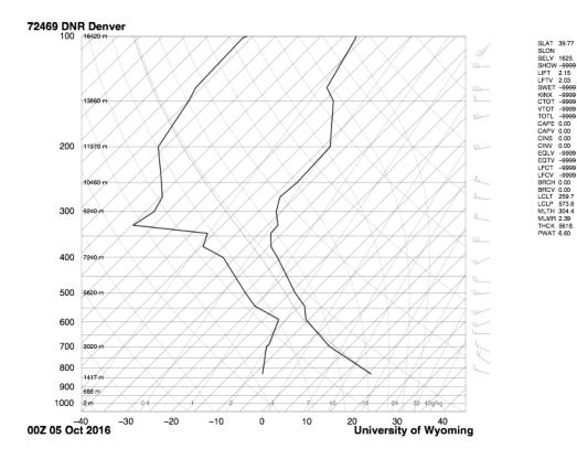
Figure 2: Skew-T plot for DIA on Oct. 4th, 6pm
