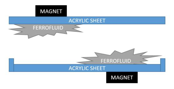
Figure 1: Apparatus setup showing the relative placement of the magnets and ferrofluid.
