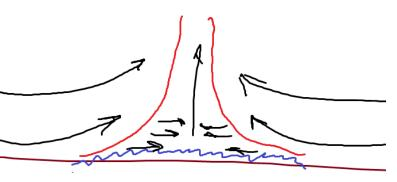
Figure 4: Cross Section of Flame Buoyancy
