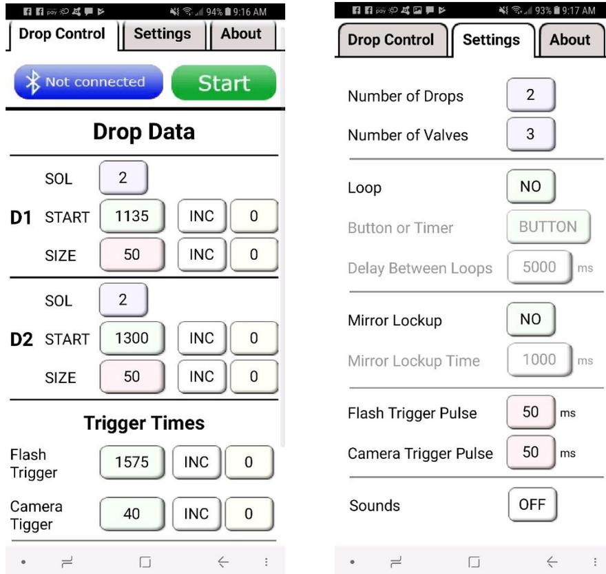
Figure 2: Dropper timing settings
