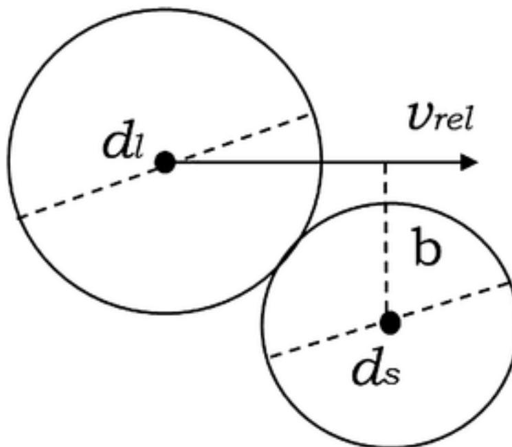
Figure 5: Droplet collision geometry
