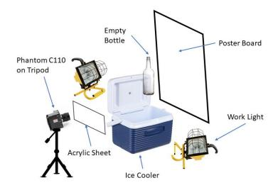
Figure 3: Setup Schematic
