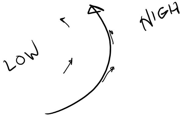
Streamlines curve because of pressure gradient. Low P is inside curve
