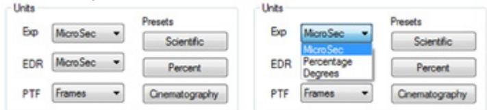
The 'Exp' unit is probably the most important unit to be set. It specifies what unit to use when setting the exposure time. You probably will want this set to micro-seconds. The other unit to set is PTF (Post Trigger Frames) covered later in this section.
