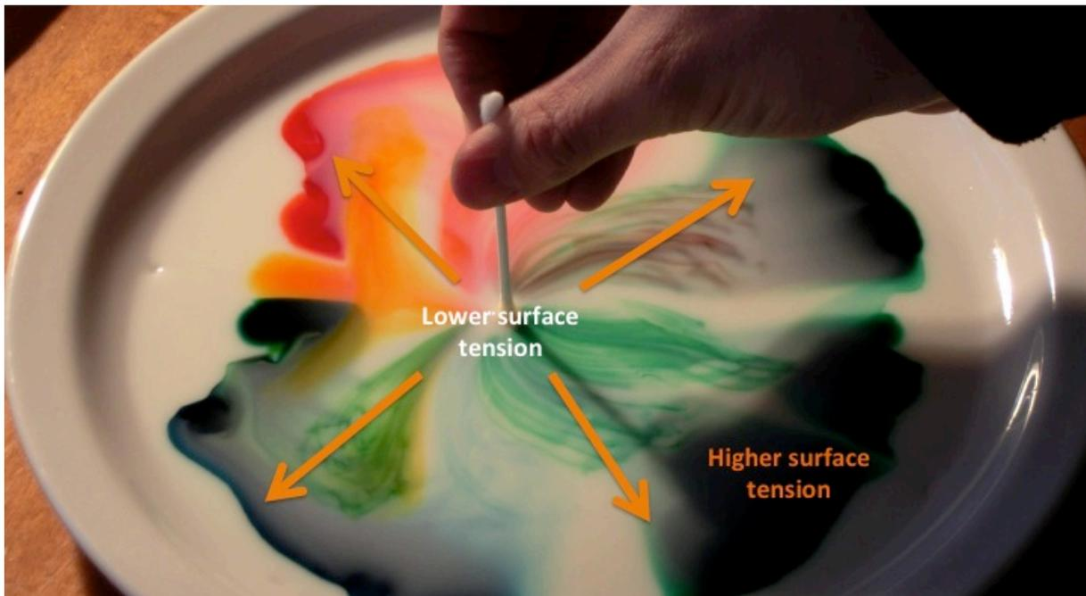
**Figure 2 - Initial interaction of the dish soap and milk**
