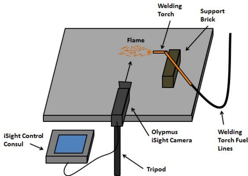
Figure 1: Experimental Setup for Welding Torch
