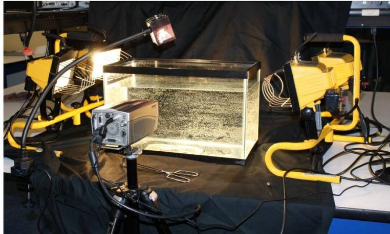
Figure 1: Fish tank, light and camera set up, Photo Courtesy of Patrick Cotter
