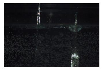
Figure 2: Still image from the video of the jets left behind after the balls were dropped. Note the lack of the jet for the center, room temperature, ball.
