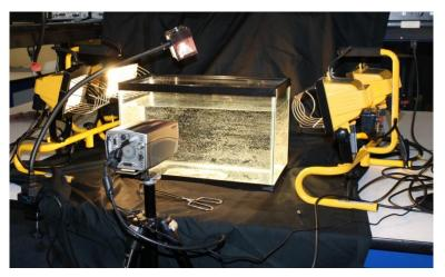
Figure 1: Fish tank, light and camera set up, Photo Courtesy of Patrick Cotter
