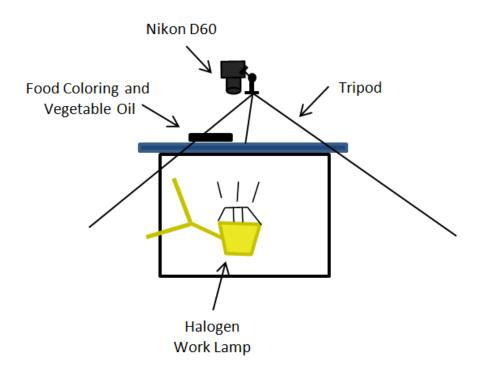
Figure 1. Photo Apparatus
