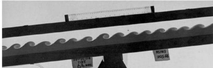
**Figure 1: Kelvin-Helmholtz instability experiment<sup>1</sup>**
