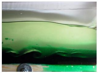
Figure 4: Kelvin-Helmholtz instability in the channel
