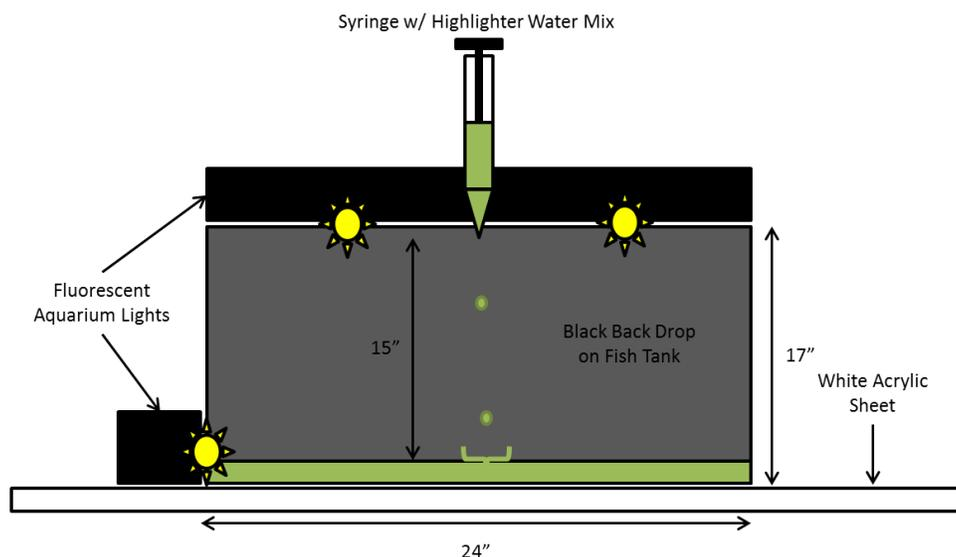
Figure 1: Flow Apparatus from Front / Camera Perspective
