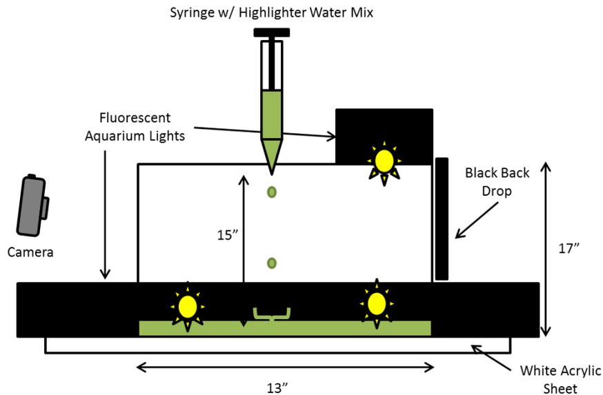
Figure 2: Flow Apparatus from Side
