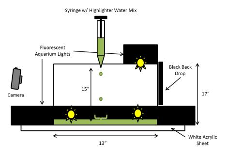
Figure 2: Flow Apparatus from Side
