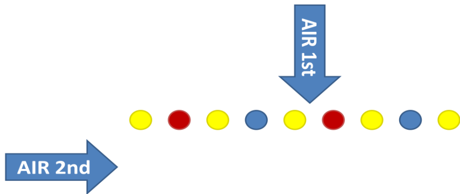
Figure 1: Set up: Drops of food coloring were dropped in a row in the pattern shown. Compressed air was blown in the directions shown by the arrows
