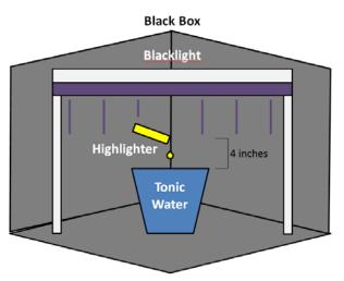
Figure 1: Flow of Apparatus
