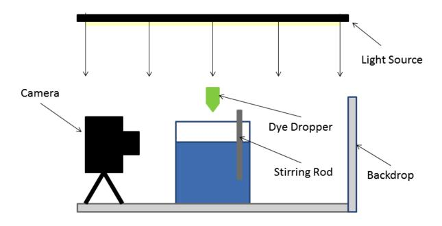
Figure 1: Experimental Flow Set-up
