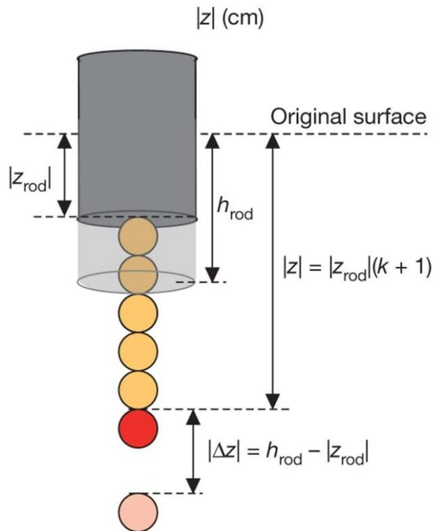
Figure 6: Compression process in an impacted shear thickening suspension where the rod first compresses suspended particles together and then translates them, compacting those below. [Waitukaitis]
