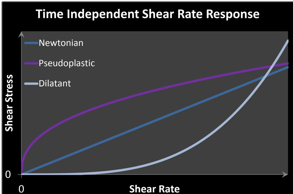
Figure 2: Shear stress as a function of shear rate for Newtonian, pseudoplastic, and dilatant fluids.
