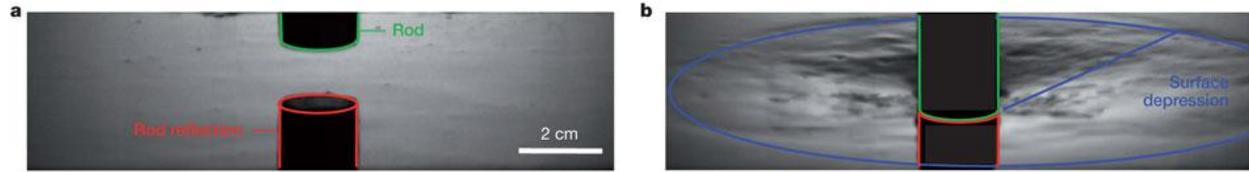
Figure 5: Example impact from experiments performed by Waitukaitis and Jaeger. a: before impact with length scale marked. b: after impact, at maximum Oobleck deflection. [Waitukaitis]
