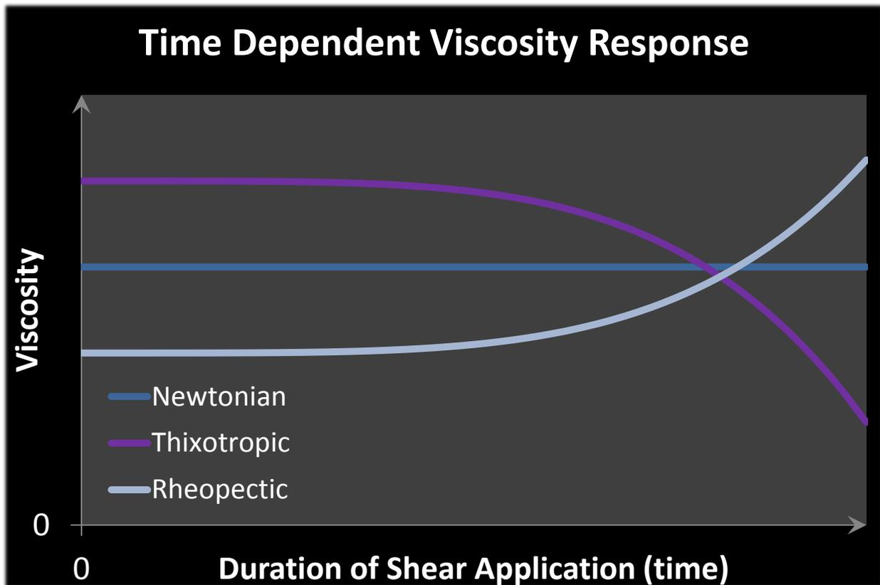
Figure 3: Viscosity as a function of time under an applied shear stress (load) for Newtonian, thixotropic, and rheopectic fluids.
