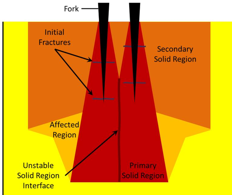
Figure 8: Schematic of theoretical solidification behavior of impact by two pronged fork.
