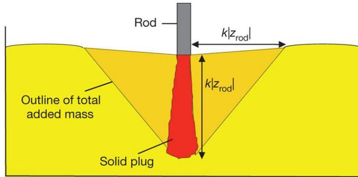
Figure 7: Schematic of the temporarily solidified region (solid plug) and the affected (added mass) region resulting from the impact of the illustrated rod. [Waitukaitis]
