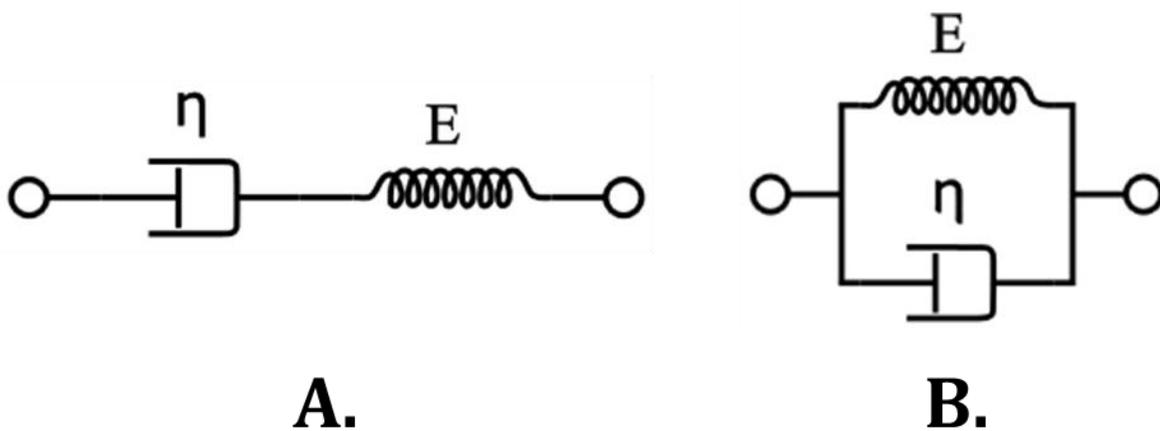
Figure 4: Spring and damper models for A. Maxwell materials, and B. Kelvin-Voigt materials
