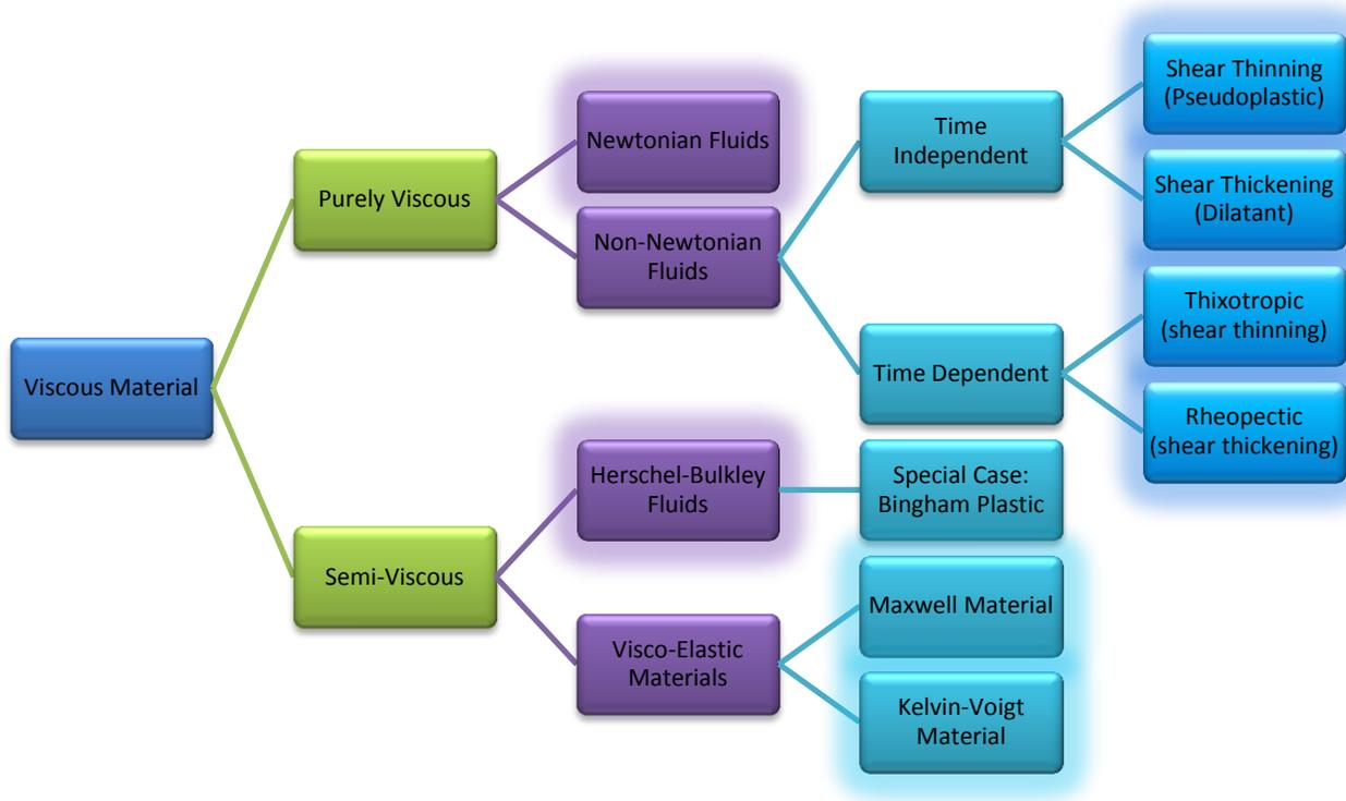
Figure 1: Break down chart for Viscous Materials. Note that all general end categories are highlighted.
